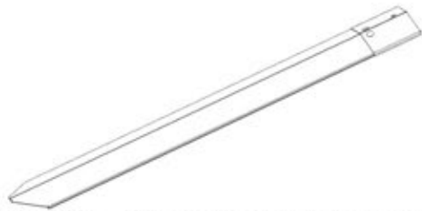
A4M01258 RIDGE CAP SPLICE ASSEMBLY (x4)
